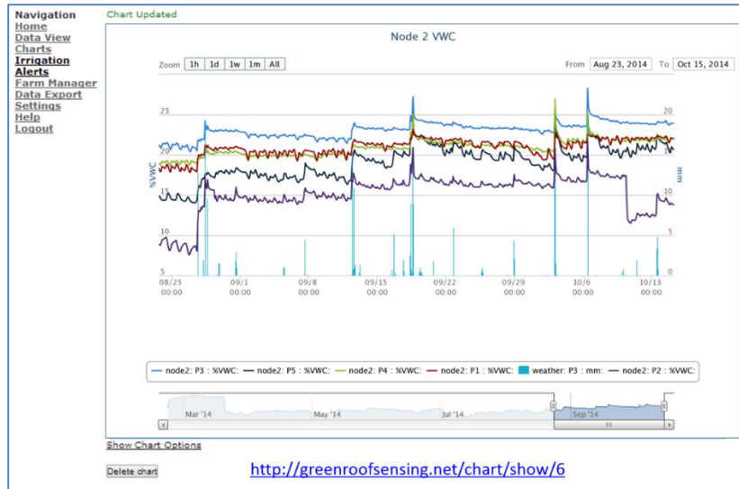
Fig 44. A Sensorweb screenshot of data from an EM50G node, showing rainfall and soil moisture dynamics
